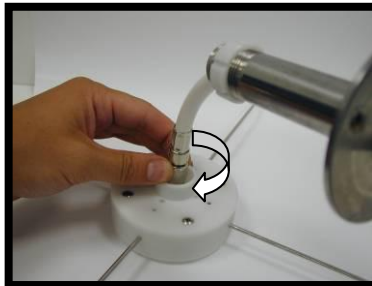
Fasten TNC cable assembly to the mating female TNC
