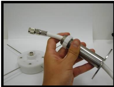
Slide wire thru mounting bracket to connect to
